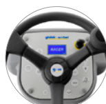
Control panel with display and water flow adjustment
